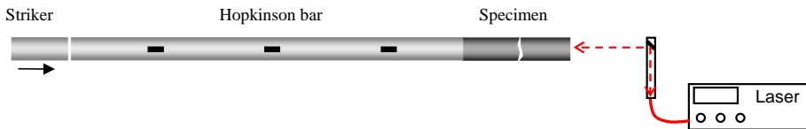
Fig.1 Principle of a modified experimental arrangement used for estimation of dynamic strength in tension
