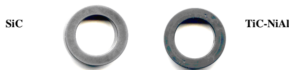
Figure 1. Sintering SiC and combustion synthesized TiC-NiAl seal ring samples.
