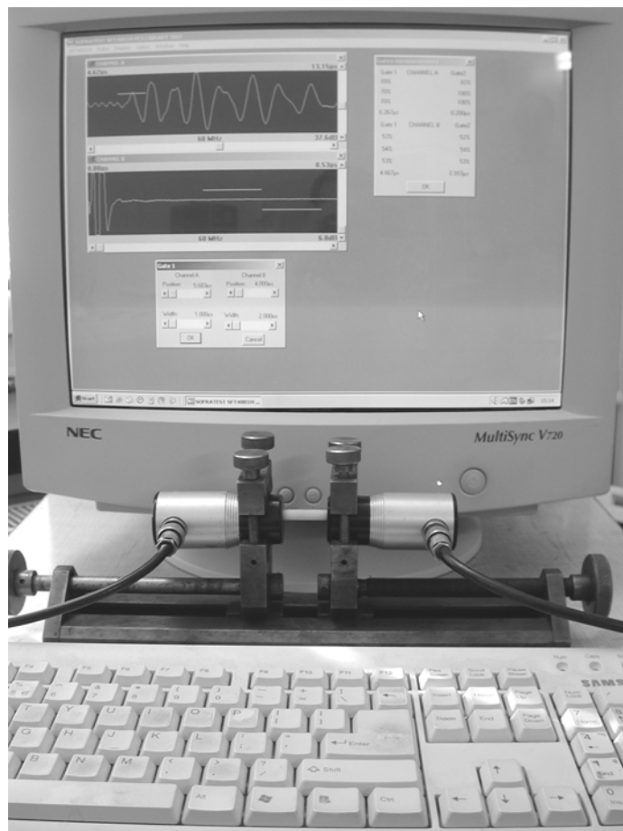
Fig. 7. Measurement of longitudinal wave in a microcore of Cervaiolle Marble (collaboration P. Gutkiewicz).
