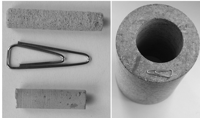
Fig. 1. Micro-cores taken out of sandstone and brick and a rock core from a mine.
